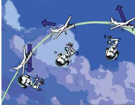
**The Head-Up Illusion** involves a sudden forward linear acceleration during level flight where the pilot perceives the illusion that the nose of the aircraft is pitching up. The pilot's response to this illusion would be to push the yolk or the stick forward to pitch the nose of the aircraft down. A night take-off from a well-lit airport into a totally dark sky (black hole) or a catapult take-off from an aircraft carrier can also lead to this illusion, and could result in a crash.
