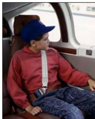
Single diagonal shoulder belts should be positioned so that the torso's center of gravity falls within the angle formed by the shoulder belt and the safety belt. Otherwise your torso may roll right out of the shoulder belt during an impact and compromise your protection.
