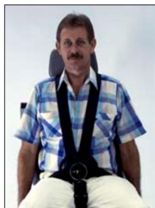
Shoulder harness systems can use dual shoulder belts or a single diagonal belt similar to those used in automobiles. The belts should not rub against your head or neck. This is uncomfortable, will discourage use of the shoulder harness, and can also cause neck injuries during an impact.
