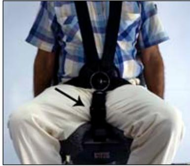
If your restraint system uses a tie-down strap, adjust it to remove all the slack when the restraint system is used. A properly installed and adjusted tie-down strap is completely safe.
